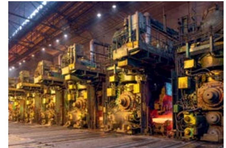
Steel Hot Rolling, Mill 2000
